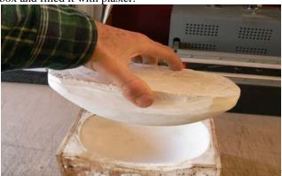
waxed up the nose cone and plunged it in. Well let me tell you wax does not make a good parting agent for plaster of Paris. So next I tried saran wrap. That worked with a couple minor wrinkles with I smoothed up. So I got a good female mold but I wanted a male to drape the acrylic over. So I tried a couple times with plastic wrap but the wrinkles were
